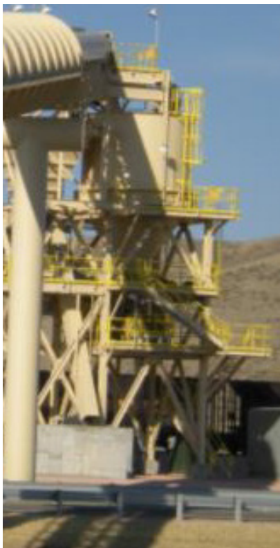
Rail Loadout Station includes MCC, Surge Bins, and Certified Belt Scales which feed spouts to railcars. Each load is metered out via these scales.
