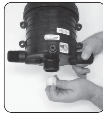
Step 3. Pry the #15 SEAL RETAINER from the injector. Pry #17 O-RING from the unit. NOTE: O-ring may still be seated at the base of the unit.
