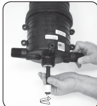
Step 7. Reinsert #51 SHAFT ASSEMBLY into body and rotate 90° to lock. Confirm the shaft is locked in by gently tugging on the shaft. Shaft should remain inserted.
