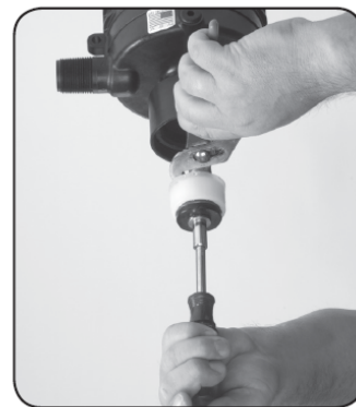
Step 3. Remove #93 CAPSCREW from the end of the shaft using a wrench and nut driver.
