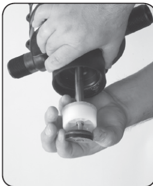
Step 4. Remove the #73 DOSAGE PISTON GUIDE and replace #44 DOSAGE PISTON and #14 O-ring.
