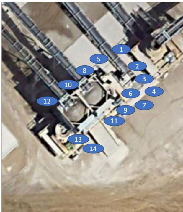
Fig. 8 Sampler placement map showing location of 14 pumps. Note the image is oriented north up
