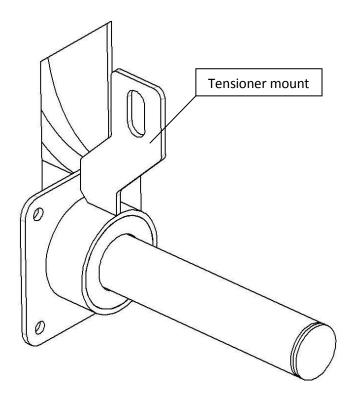
a. Attach the tension arm, threaded rod, and tension spring. Tighten the arm to the pole. Spring should face the back of the head chute, away from the headpulley.
