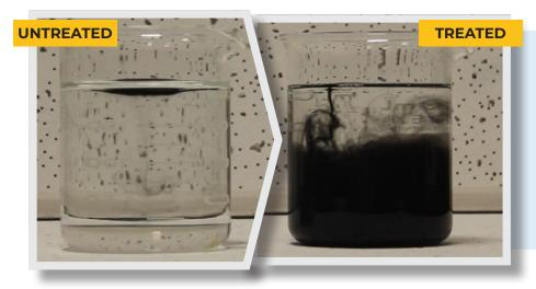
This demonstration shows how the BT-205W surfactant is able to alter the surface tension of water, effectively overcoming the hydrophobic properties of petroleum coke dust and causing it to submerge in treated water, unlike in plain water where the dust remains suspended on the surface.
