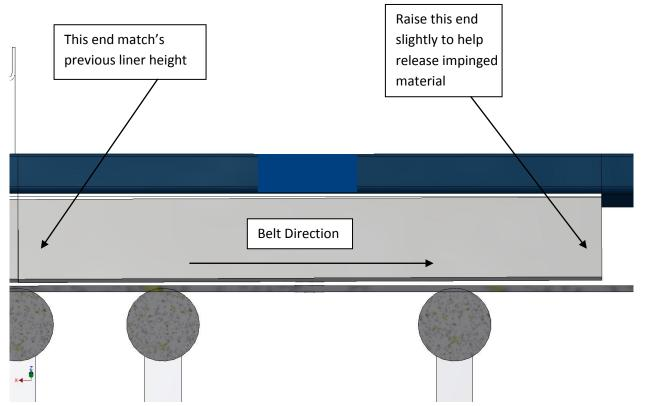
7. Install chosen Rubber Seals allowing them to make contact with the belt.
